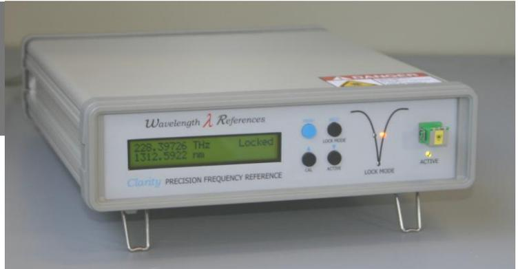
The Wavelength References Clarity laser family locks a laser emission to a molecular absorption line. The instrument drives a semiconductor laser in a unique configuration that creates superb frequency stability traceable to a physical constant and thus forms primary frequency standard. The Clarity can lock to several transitions and materials, check for availability.
